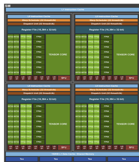
Figure 3. The architecture of SM in NVIDIA’s Ampere GPU from NVIDIA’s official whitepaper [12].
