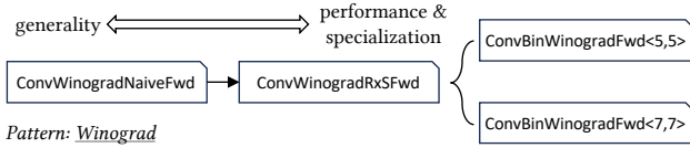
Fig. 4. Generality-performance trade-offs for Winograd solutions. Specialized solutions are more performant but applicable for specific problems, while generic solutions can be applied to more problems but are less efficient.
